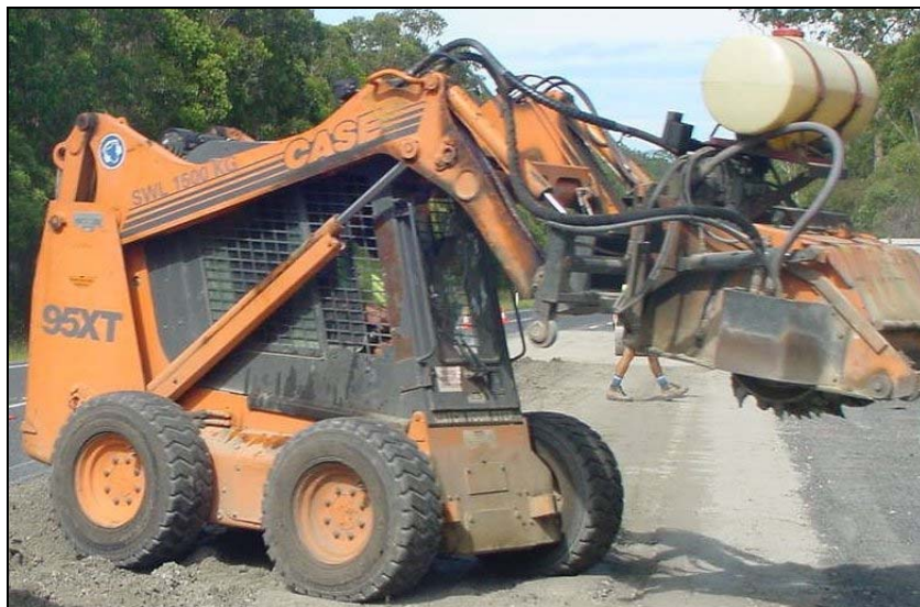
Figure 1 View of skidsteer patrol patcher.
