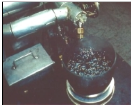
Figure 5 Foamed bitumen being produced in the laboratory.
