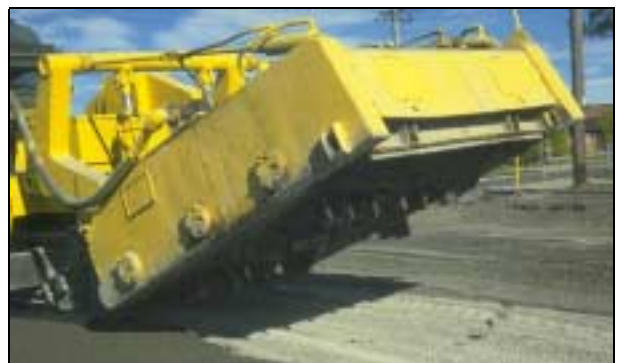
Figure 3 A P&H machine with a triple rotor system (CIRCA 1978).
