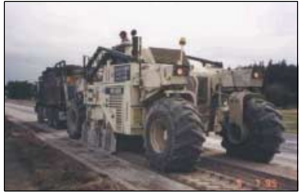
Figure 1 A RS500 reclaimer/stabiliser with a 325kW engine and single rotor system.
