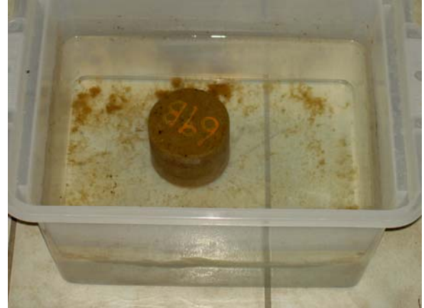
This lime treated subgrade sample has been soaking for nearly 12 months. In comparison, the untreated sample fell apart in a few hours.
