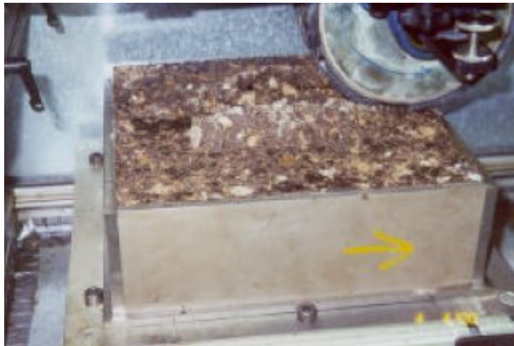
Figure 6 Deflection results from wheel rutting test of foamed bitumen stabilised material (Ramanujam, 2000).
