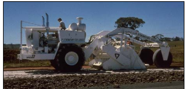
Figure 1 Conventional stabiliser. Note the centrally mounted mixing chamber.
