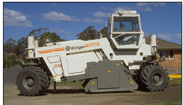
Figure 1. Dedicated reclaimer/stabiliser for insitu foamed bitumen stabilisation.
