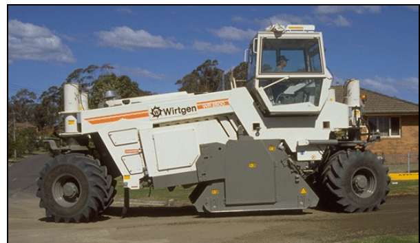
Figure 1. Dedicated reclaimer/stabiliser for insitu foamed bitumen stabilisation.
