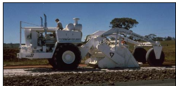
Figure 1 Conventional stabiliser. Note the centrally mounted mixing chamber.
