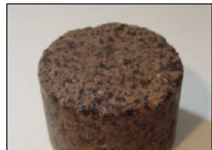
Figure 3 The foamed bitumen stabilised material has the colour of the dominant parent aggregate.
