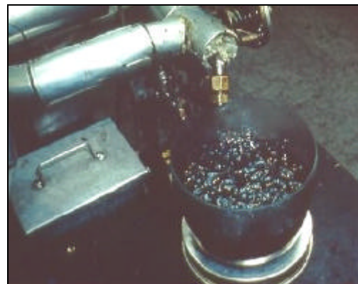
Figure 5 Foamed bitumen being produced in the laboratory.
