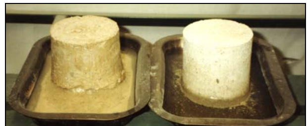
Figure 2 A view of a pavement material sample unstabilised (left) and stabilised with DPP (right) subject to soaking in water for 24 hours.
