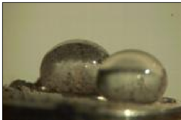
Figure 1 A view of a water droplet failing to penetrate the surface of a DPP stabilised material.
