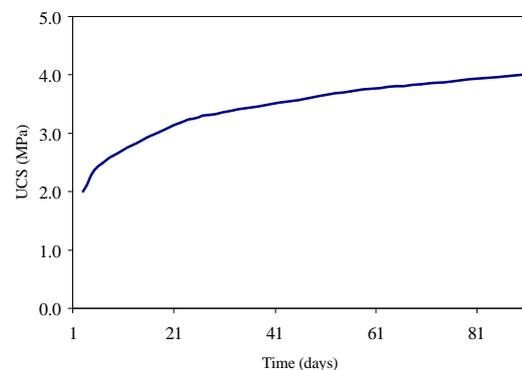
**Figure 2** As a binder cures the stabilised layer develops strength over time.
