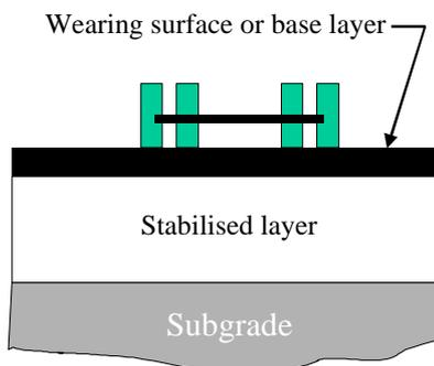
**Figure 1** A view of a typical cross-section through a stabilised pavement.
