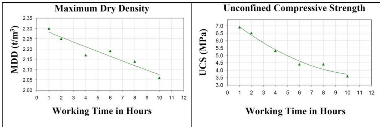
**Figure 2:** Working time charts for MDD and UCS with working times of 3.25 and 2.5 hours respectively with 4% binder content (BCSC, 2005). Tested to RTA R75 specification.
