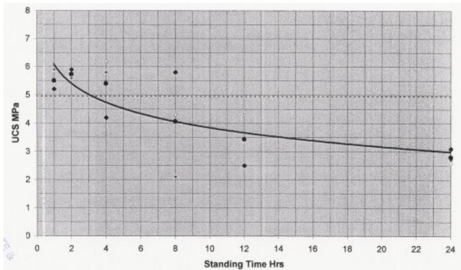
**Figure 6:** Plot of UCS versus standing time for a slow setting binder and crush rock.
