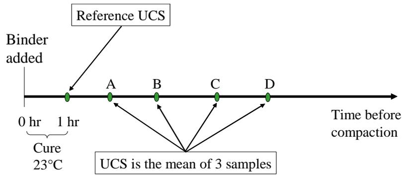
**Figure 3:** Timing of the compaction (standing time) of the samples after the commencement of mixing the binder and pavement material.
