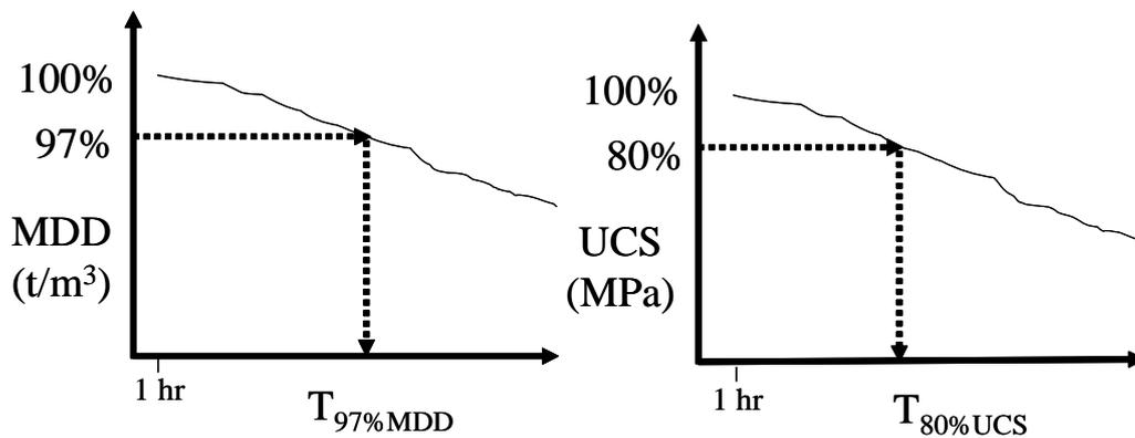
**Figure 1:** The RTA definition is based on testing the material for density and compressive strength.
