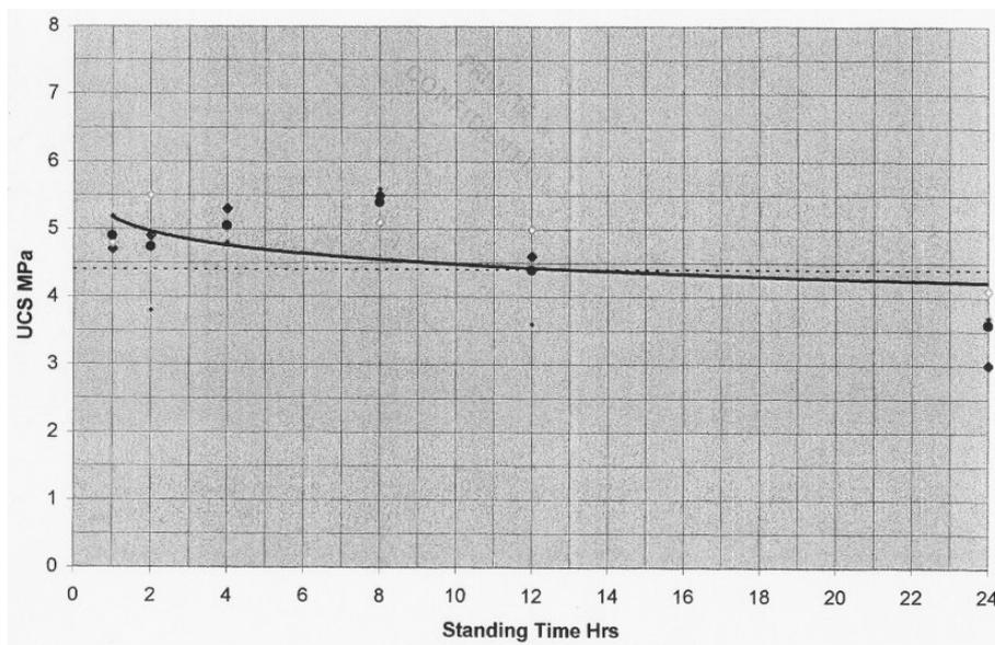
**Figure 5:** Plot of UCS versus standing time for a slow setting binder and crush rock showing the 'flatness' of the curve.
