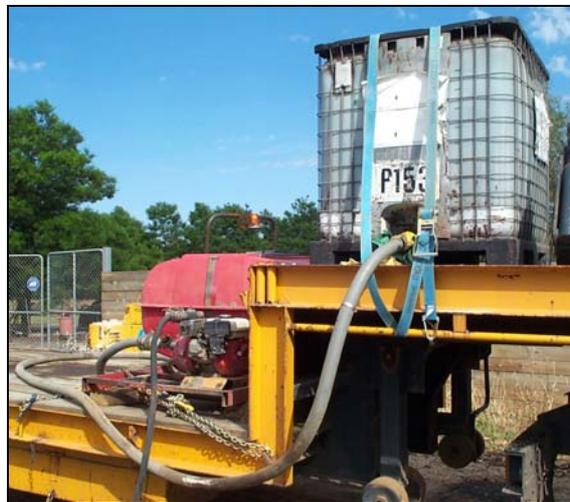
**Figure 8** Intermediate bulk containers for chemical liquid binders.
