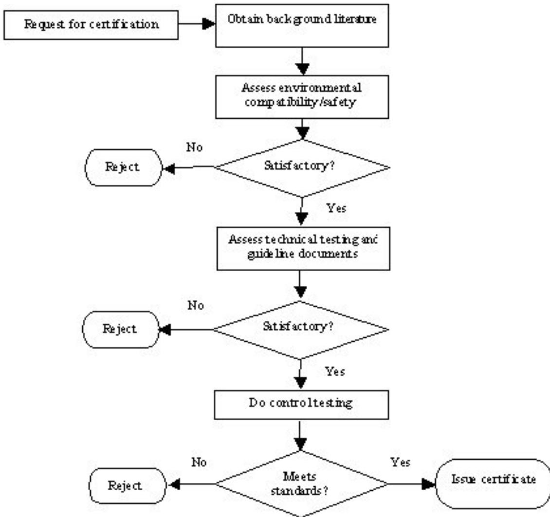
**Figure 3** Recommended certification procedure from work by CSIR Transportek (Jones,2003).
