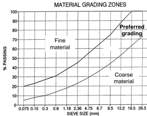
**Figure 4** Good particle size distribution is required to achieve strength and durability (Austroads, 2002).
