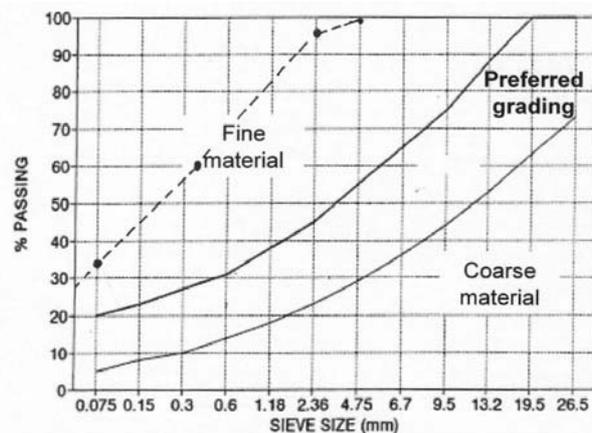
**Figure 5** Particle size distribution (dashed line) of prior stream gravel from SW region of NSW (Kok, 2003).
