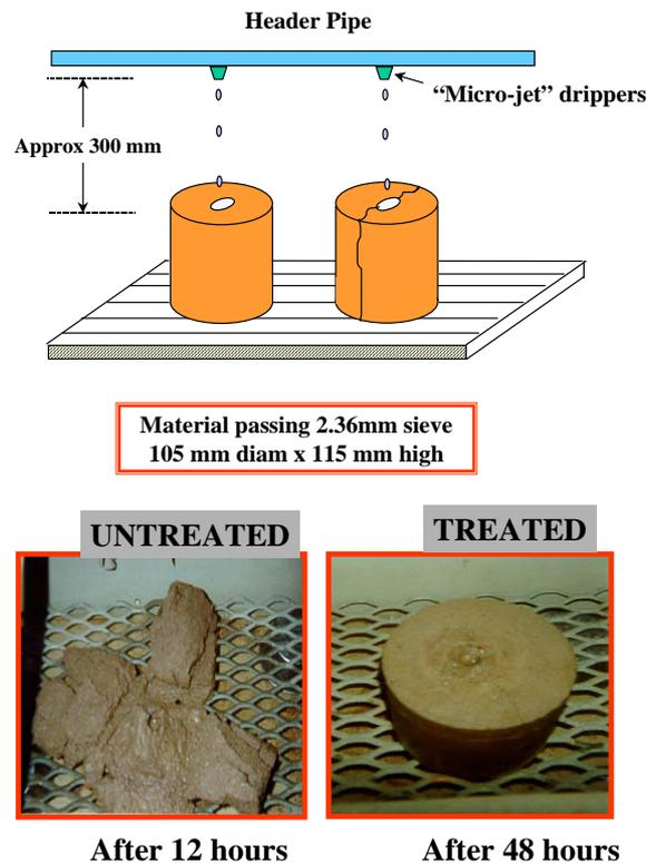
**Figure 6** Transport SA saturation test apparatus (Austroads, 2004).
