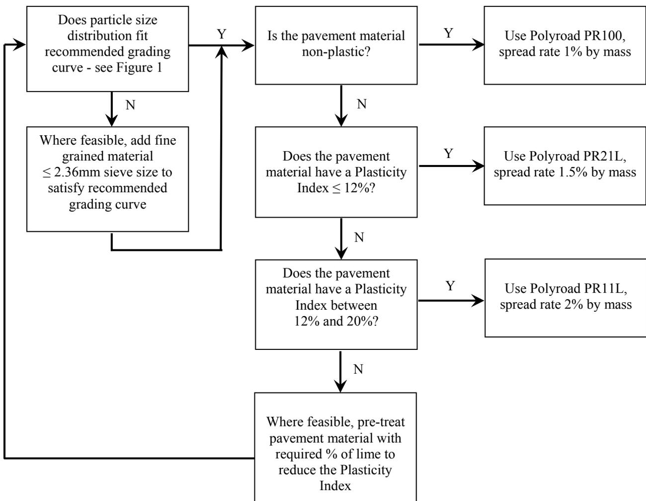
Figure 3 Mix Design Selection Flowchart
