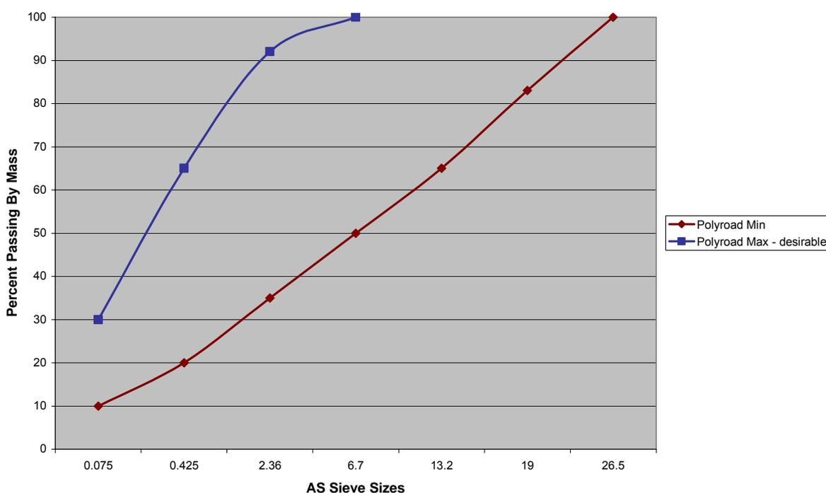
Figure 1 Recommended Particle Size Distribution for Insoluble DPP Stabilisation
