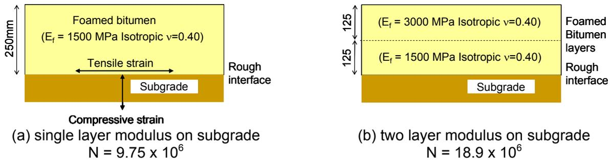
**Figure 1** The number of repetitions to fatigue cracking for a single and double modulus layer using the design model in this paper.
