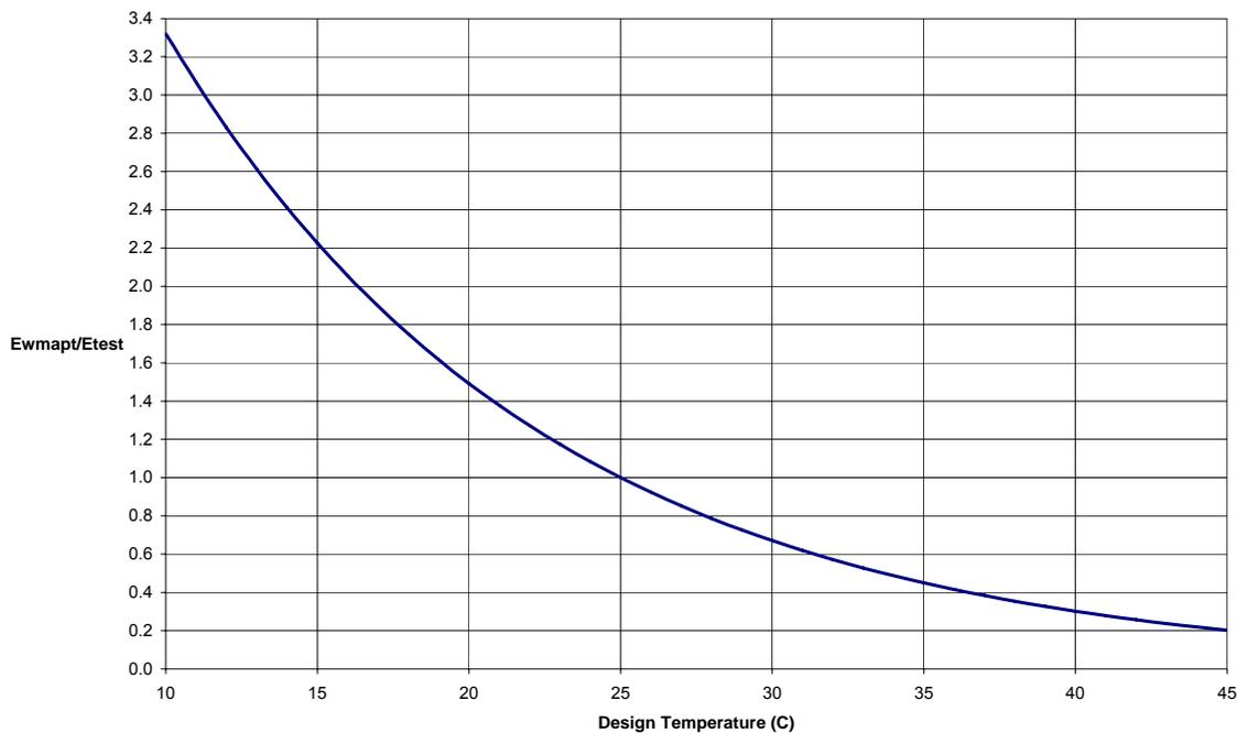
**Figure 2** Ratio of modulus at WMAPT ( $E_{WMAPT}$ ) to the modulus from Standard Indirect Tensile Test ( $E_{test}$ ) for conventional asphalt mixes only. (Austrads, 2004a)
