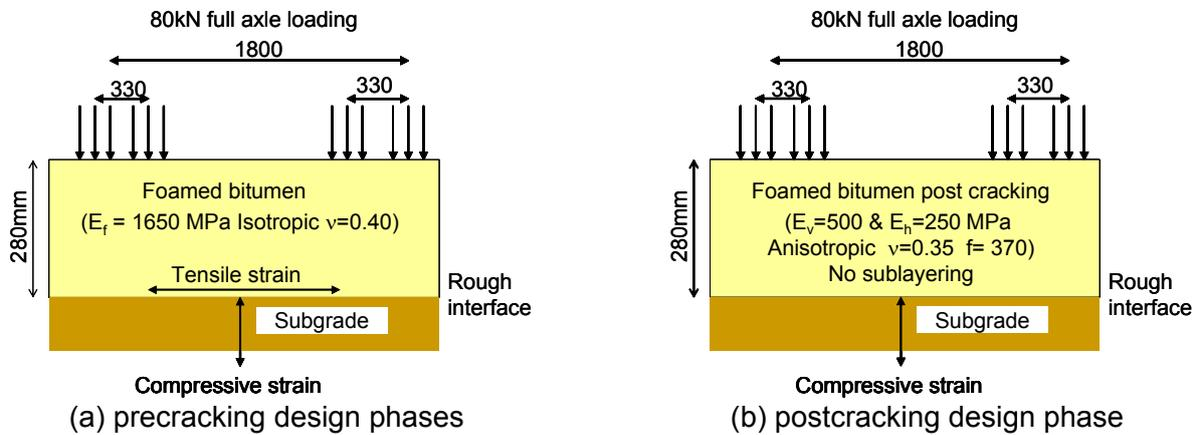
**Figure 3** Design example as modelled in CIRCLY 5 for precracking and postcracking design phases.
