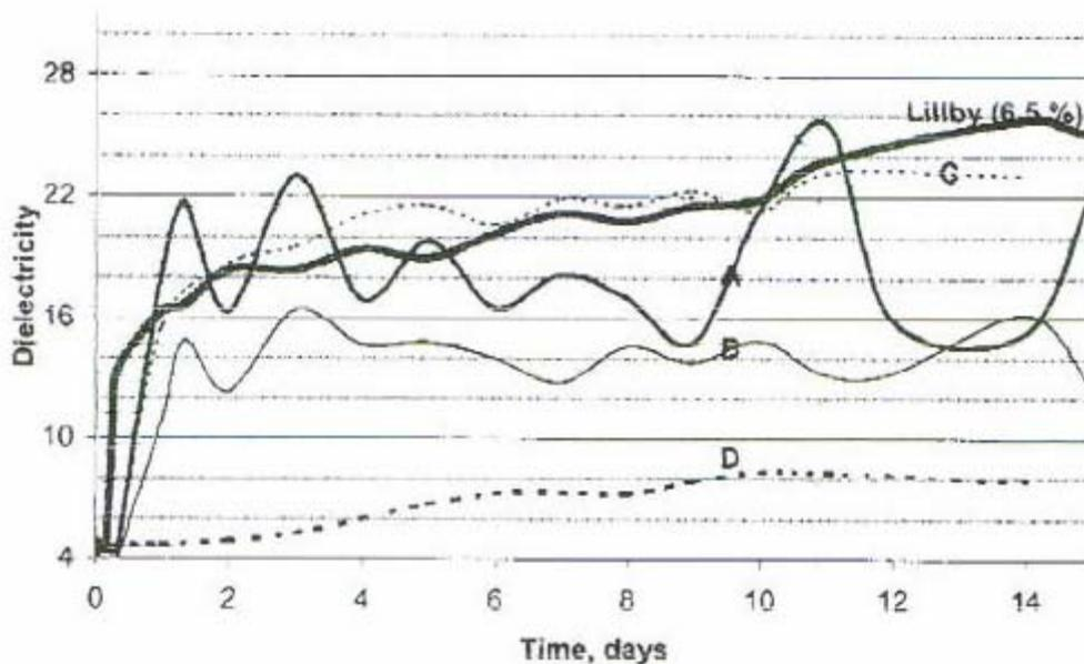
**Figure 9** Dielectricity results for Lillby crushed aggregate.
