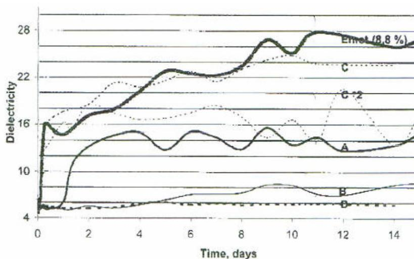
**Figure 10** Dielectricity results for Emet crushed aggregate.
