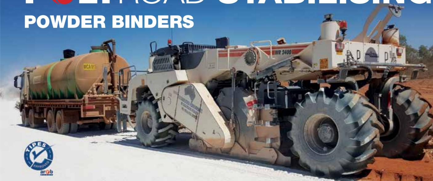
Polyroad is an extremely useful stabilisation binder, enabling us to extend the range of materials suitable for stabilisation, and thereby conserve a greater quantity of natural materials. Being a dry powder polymer (DPP) Polyroad is insoluble in water and most importantly does not degrade or leech in the field. When stabilising with Polyroad
