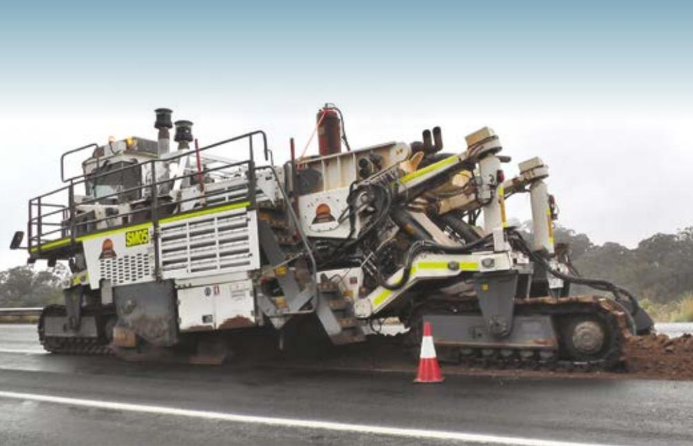
This was the first time a surface miner had been used on the Roads and Maritime Services road network in New South Wales. It was an innovative pre-treatment solution, used prior to traditional stabilisation using a centrally mounted mixer with moisture control.
