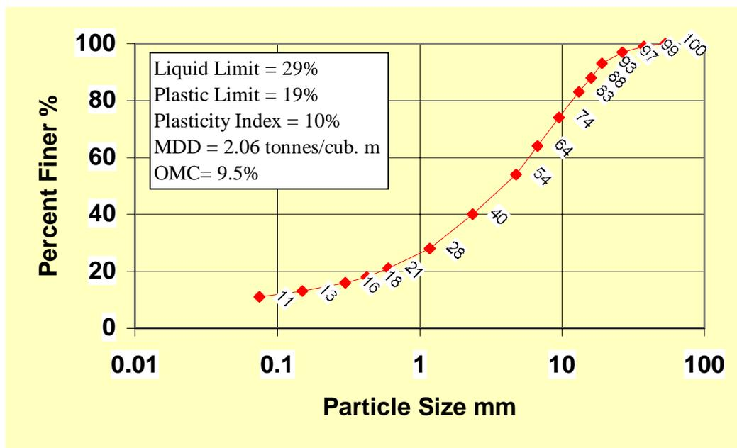
Figure 2 Sheeting Material Post Compaction Classification Properties
