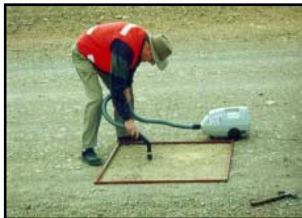
*Figure 6 Removal of loose Surface Material*
