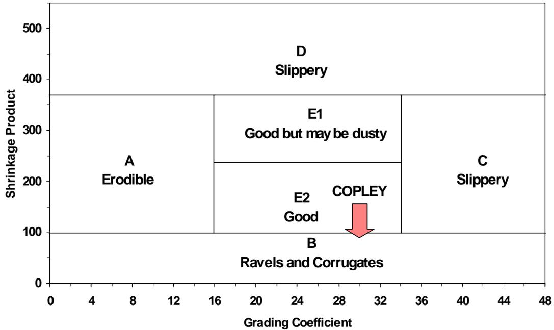
Figure 11 Grading/Plasticity and Unsealed Surface Performance<sup>[4]</sup>
