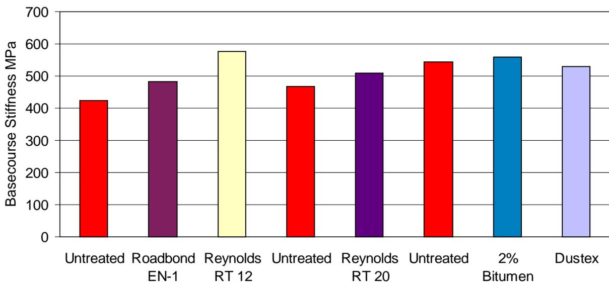
*Figure 4 Basecourse Stiffness (Elmod back-calculated Resilient Modulus)*
