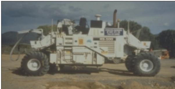
Figure 5 View of common reclaimer and stabiliser with 500hp engine.
