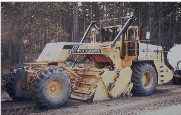
Figure 1 Conventional-sized reclaimer/stabiliser.
