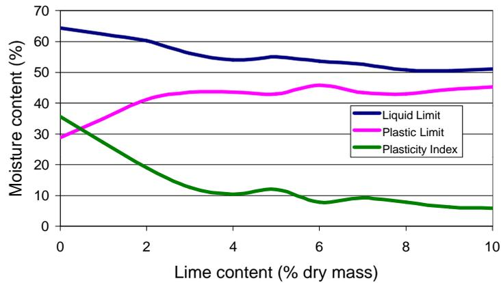
**Figure 1** Lime content versus liquid limit, plastic limit and plasticity index for Killarney road trial pavement.
