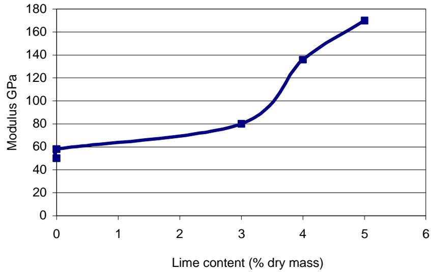
**Figure 3** Modulus data (derived from CIRDEF after 6 months) from the Killarney Road trial.
