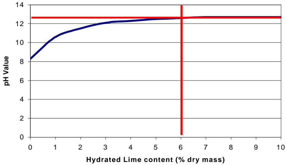
**Figure 6** Lime content (based on lime demand) versus pH value for Cunningham Highway, Warwick trial pavement.
