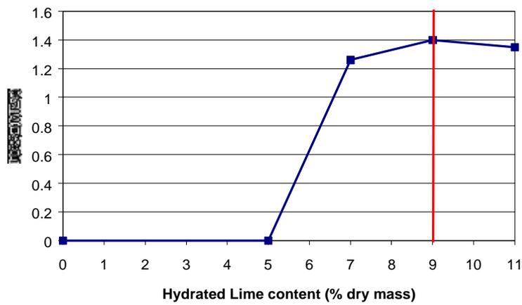
**Figure 7** Lime content versus 28-day UCS based on Thompson's method for Cunningham Highway, Warwick trial pavement.
