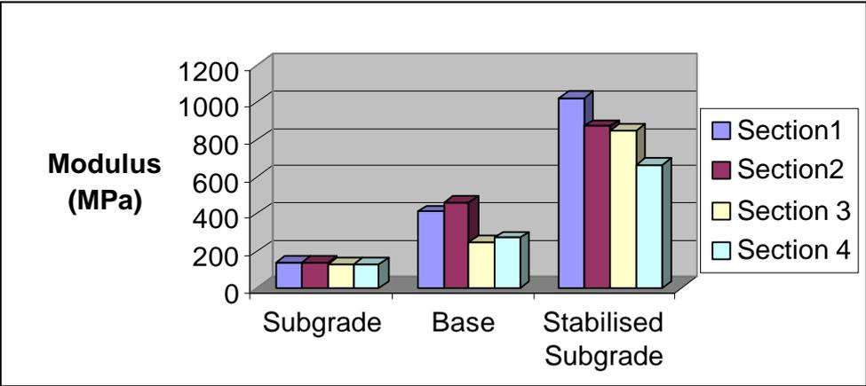
**Figure 9** Back analysed modulus data at 6 weeks.
