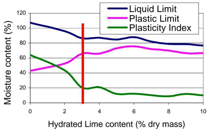
**Figure 5** Lime content, based on lime fixation, versus liquid limit, plastic limit and plasticity index for Cunningham Highway, Warwick.
