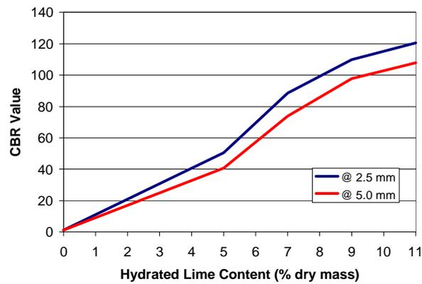
**Figure 8** Lime content versus laboratory soaked CBR values.
