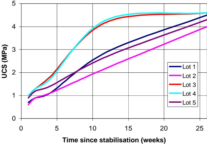
**Figure 10** UCS data – cylinders taken during stabilisation process.
