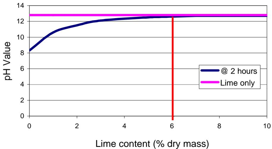
**Figure 2** Lime content versus pH value based on Eades and Grim Test method (Killarney road trial pavement).
