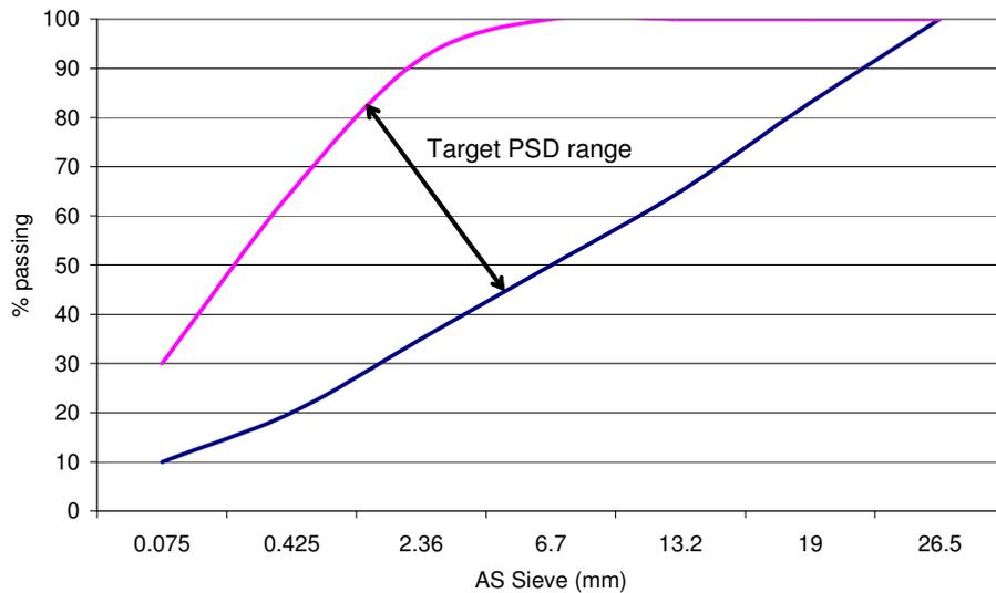
**Figure 4** Suggested particle distribution range for Polyroad binders.
