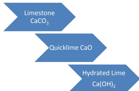
Figure 1 The Lime Cycle
