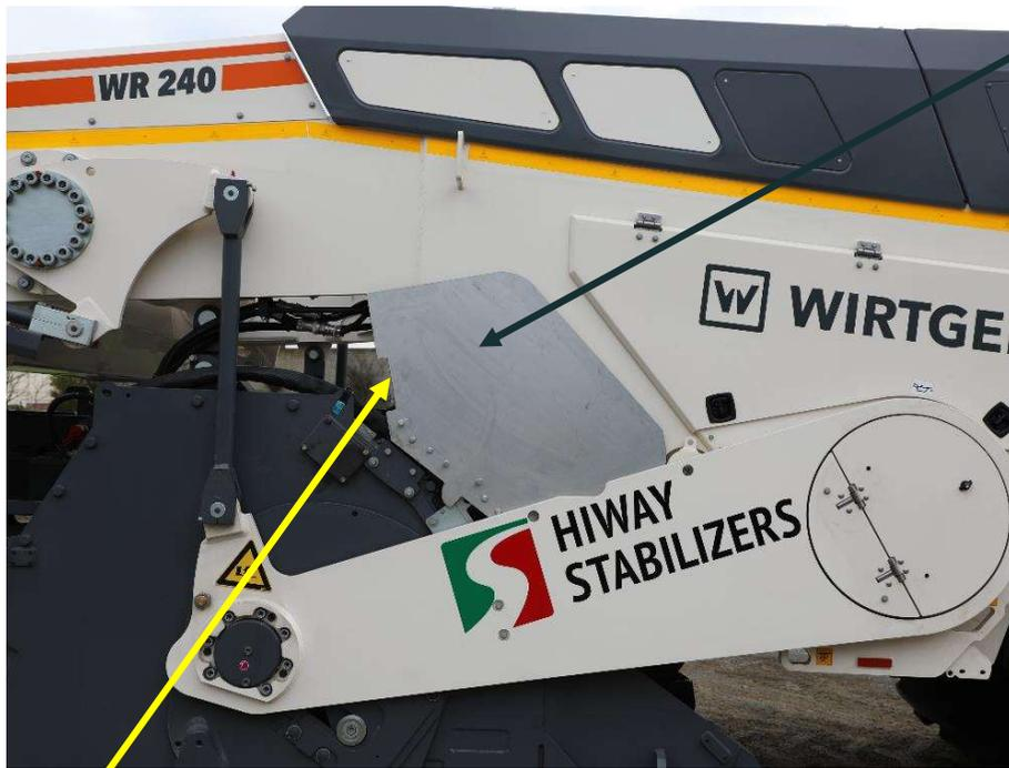
Guard fitted to provide a barrier for uncontrolled release of bitumen
